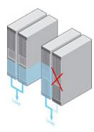
To achieve the highest level of availability and to power critical utilities, NETYS RT UPS modules above 3 kVA can be configured for 1:1 redundancy.
