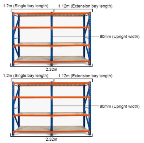
\*Based on a 2.4m shelving unit. The same principle can be applied to 1.2m, 1.5m and 2m shelving units to work out precise length.
