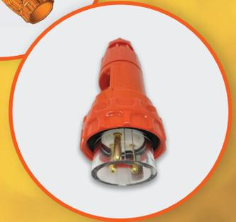
The 4Cabling industrial power plug is a movable connector attached to an electrical power cord. This new patent pending\* design isolates the wire within the housing structure which allows the measurement of the current in a safe and easy manner using a clamp-on meter.
