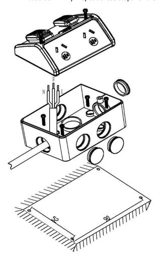
3.2 For the recess mounted option, assemble on the wall, fix the cover, and then glue the edges in place. For wiring, refer to the previous instructions.
