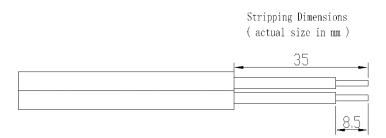
4. Wire as indicated below. Please note that the 'line' marking is the connection end, and the 'load' marking is the load end. **Connection end "L" must match load side "L".**
