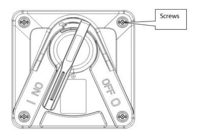
2. Install the base as below, tightening the four screws and using glue to seal.
