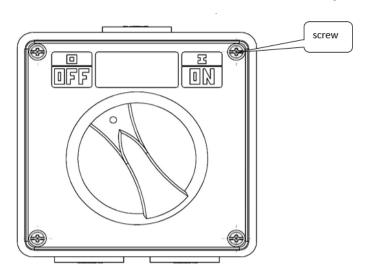
2. Install the base as below, tightening the four screws and using glue to seal.
