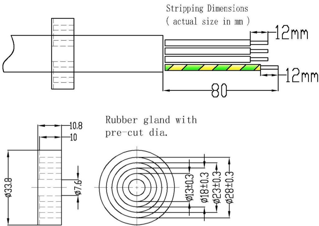
2. Assemble per the diagram below, being careful of seal direction.
