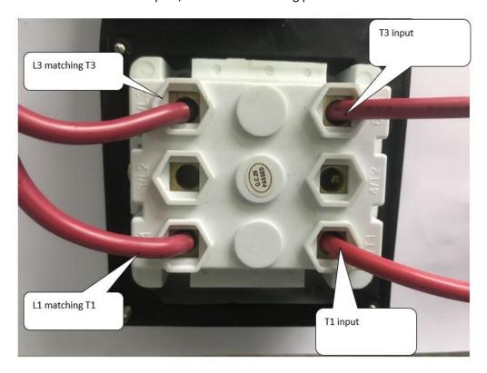
a. For models 040.000.0140, 040.000.0205-206 T1, T2 and T3 = inputs, L1, L2 and L3 = matching phase line for T1, L2 and T3
